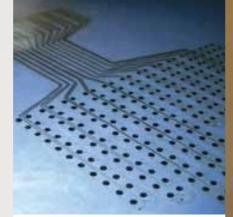
Micromachined electrode array
