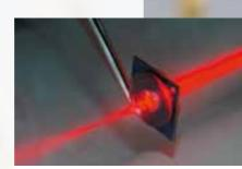
Adaptive lens with piezo actuator
