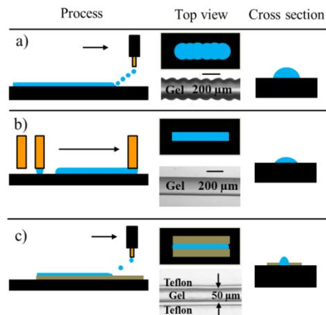
Figure 1: a) Periodic droplet jetting to produce linear structures on planar substrates. b) Semi-contact writing method. The nozzle of a dispenser is moved close to the substrate ( $\sim 100 \mu\text{m}$ ). The ejection of a single droplet establishes a capillary bridge between nozzle and substrate. Complex fluidic structures are generated due to capillary flow by controlled displacement of the substrate along the x-y-plane. c) Combined method of the SCW-technology and droplet jetting.
