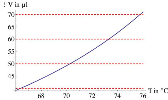
Figure 1: Calculation of temperature (intersection of blue and red curves) at which 40  $\mu\text{l}$ , 50  $\mu\text{l}$ , 60  $\mu\text{l}$ , and 70  $\mu\text{l}$  (red dotted lines), respectively, of volume expansion  $\Delta V(T)$  of an initial saturated air volume  $V_1 = 79.7 \mu\text{l}$  at room temperature  $T_1 = 24.4 \text{ }^\circ\text{C}$  and atmospheric pressure  $p_{\text{atm}} = 100.6 \text{ kPa}$  is expected.
