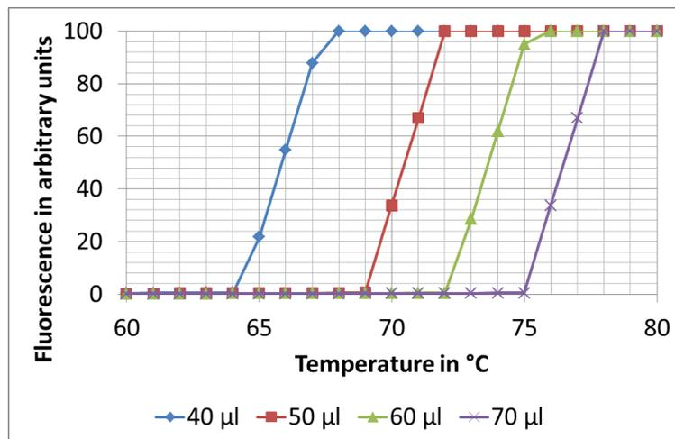
Figure 3: Sudden fluorescence signal increase during melt curve analysis inside the detection chamber of the fluidic temperature measurement system (FTMS) with a 40 µl (blue), 50 µl (red), 60 µl (green), and 70 µl (purple) siphon volume, respectively, at a distinct temperature.
