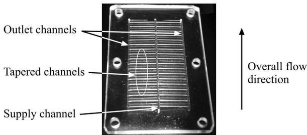
Figure 4. Photograph of one of the transparent test samples
