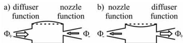
Figure 1: Nozzle-diffuser pump with the inlet on the left side and the outlet on the right in a) supply mode and b) pump mode causing a net-flow towards the right side.
