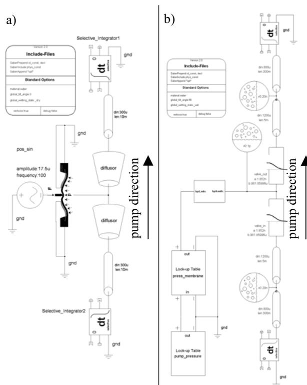
Figure 4: Model setup of a) the nozzle-diffuser pump [4] with a piezoelectric actuation and nozzle-diffuser valves [9] and b) the flap valve pump [6] with a pneumatic actuation.
