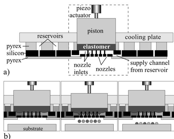
**Figure 1.** Schematic view of the TopSpot Vario set-up (top) and working principle (bottom)
