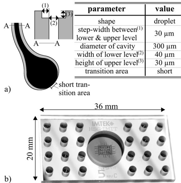
**Figure 3.** Optimized printhead design **a)** suggestion rules for 2-level TopSpot Vario nozzle inlets and nozzle inlet channels [5] **b)** TopSpot Vario printhead with implemented 2-level microfluidic structures
