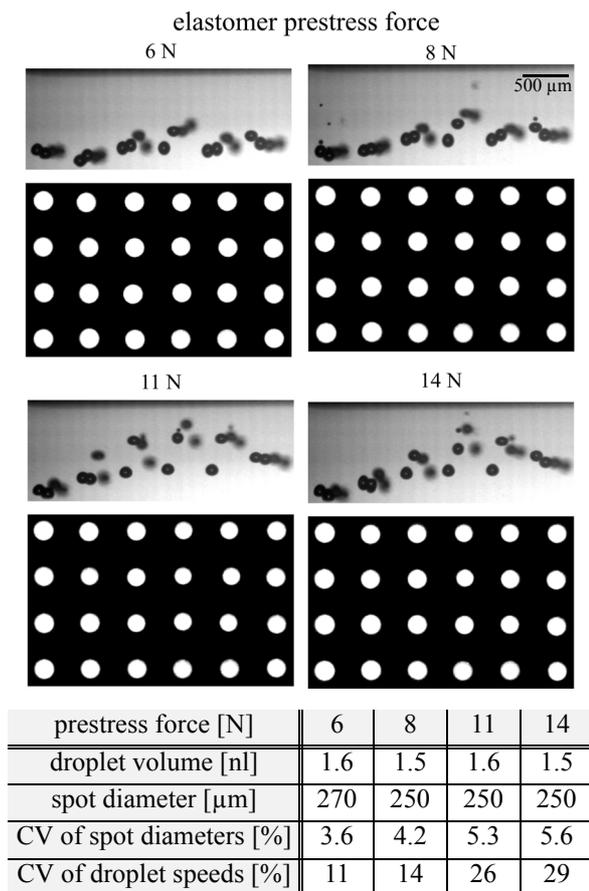
**Figure 5.** Influence of elastomer prestress force on droplet and spot homogeneity respectively. Top pictures show camera records of ejected droplet arrays and bottom pictures show resulting microarrays recorded by the fluorescence scanner. The table lists mean droplet volume and spot diameter of all droplets/spots in one array as well as the CVs of droplet speed and spot diameters of all droplets/spots of one array.
