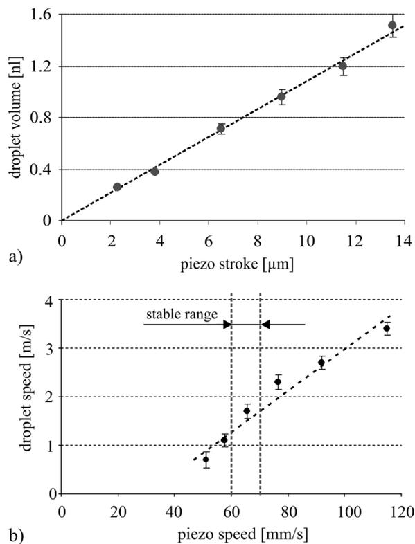
**Figure 4.** Influence of piezo movement on droplet volume and speed **a)** droplet volume versus piezo stroke. Error bars represent the CV of 5 % of mean droplet volume of all 24 droplets of one array between the experiments **b)** droplet speed versus piezo speed. Error bars represent CV of droplet speeds of all 24 droplets in one array.
