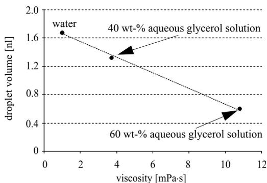
**Figure 6.** Droplet volume versus liquid viscosity at a constant piezo stroke of 13  $\mu\text{m}$
