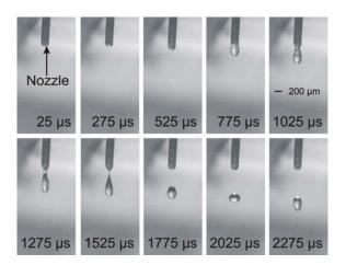
Fig. 3: (A) Pictures of the droplet ejection from  $PipeJet^{TM}Tip$ .
