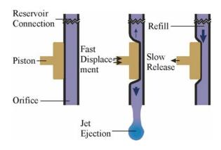
Fig. 2: Dispensing principle scheme: A piezo actuated piston squeezes the polymer tube and generates a pressure forcing the ejection of a droplet. Slow release of the piston allows capillary filling of the tube.
