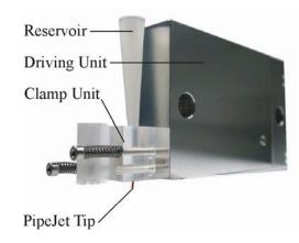
**Fig. 1:** (A) The disposable PipeJetTip<sup>TM</sup> consists of a standard pipette tip that can be used as reservoir and a polymer tube with a diameter of 500  $\mu$ m. (B) The PipeJet<sup>TM</sup> module features a clamp unit for fixation of the tip and a driving module with integrated piezo-driven actuator.
