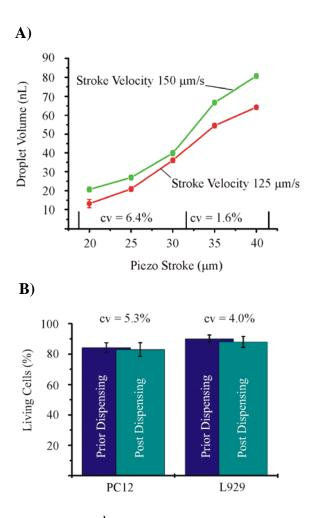
Fig. 4: (A) Correlation between the DMEMSdroplet volume and the piezo stroke for two different stroke velocities. The droplets exhibit high reproducible volumina from 10 nL to 80 nL. (B) Comparison of the percentages of living cells prior to and after dispensing. Only a small fraction of both tested cell lines ares affected by the dispensing process.
