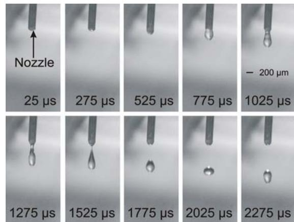
**Fig. 3:** (A) Pictures of the droplet ejection from PipeJet™Tip.
