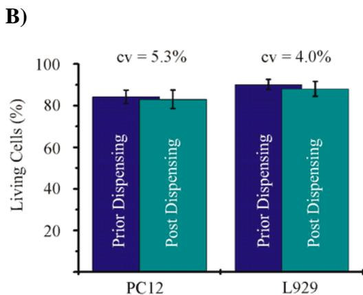
**Fig. 4:** (A) Correlation between the DMEMS-droplet volume and the piezo stroke for two different stroke velocities. The droplets exhibit high reproducible volumina from 10 nL to 80 nL. (B) Comparison of the percentages of living cells prior to and after dispensing. Only a small fraction of both tested cell lines are affected by the dispensing process.
