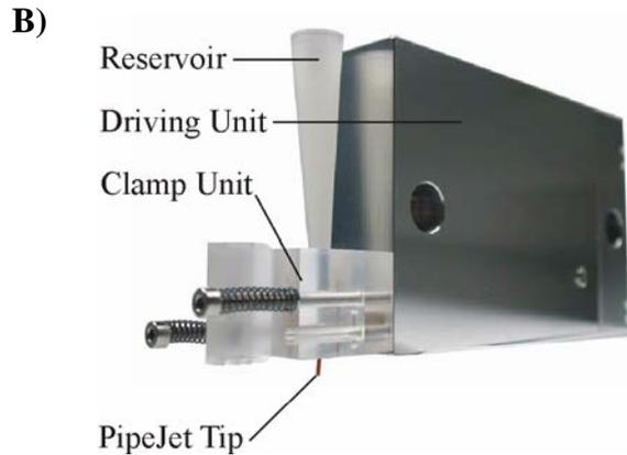
**Fig. 1:** (A) The disposable PipeJetTip™ consists of a standard pipette tip that can be used as reservoir and a polymer tube with a diameter of 500  $\mu\text{m}$ . (B) The PipeJet™ module features a clamp unit for fixation of the tip and a driving module with integrated piezo-driven actuator.
