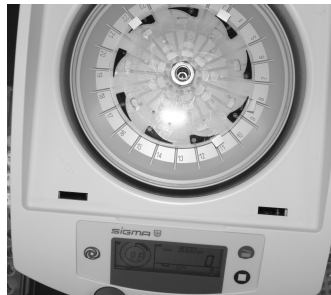
Figure 3: Experimental Setup. Microfluidic DNA-extraction disk on standard laboratory centrifuge.
