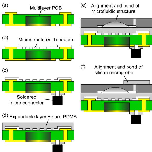
Figure 5: Schematic illustration of fabrication and assembly of the different components of the NeuroMedicator.
