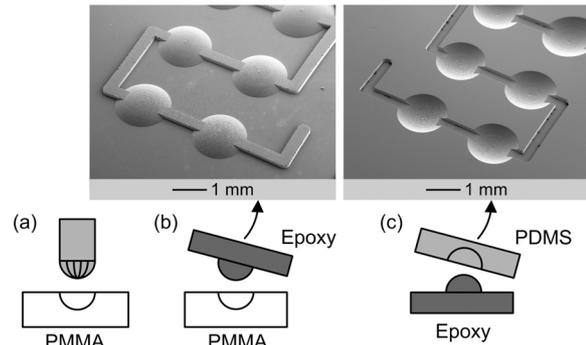
Figure 3: Three-step fabrication process of the microfluidic structure. (a) Milling of a positive PMMA master, (b) casting of a negative epoxy mould, and (c) PDMS replica moulding of the fluidic structure.
