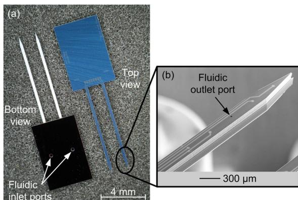
Figure 4: Fabricated fluidic silicon microprobes. (a) Top and bottom view of microprobes. (b) SEM picture of the probe tip.
