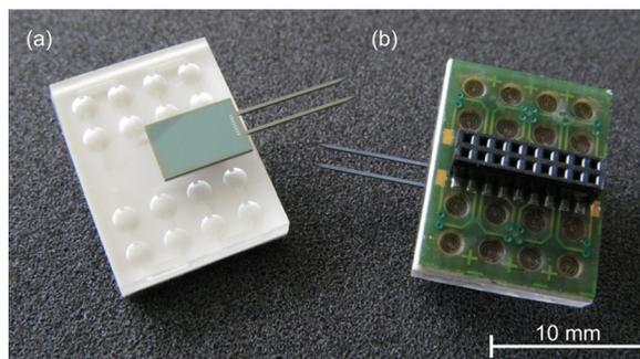
Figure 6: Assembled NeuroMedicators showing (a) the top side with the fluidic chambers and the microprobes as well as (b) the bottom side with the electrical connector.
