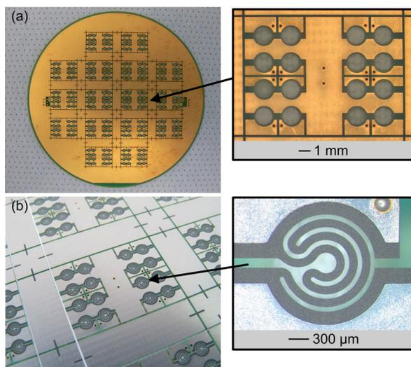
Figure 2: Thin film fabrication of microheaters. (a) Multilayer PCB 100-mm-disc. (b) Fabricated microheaters after deposition and etching of Ti.
