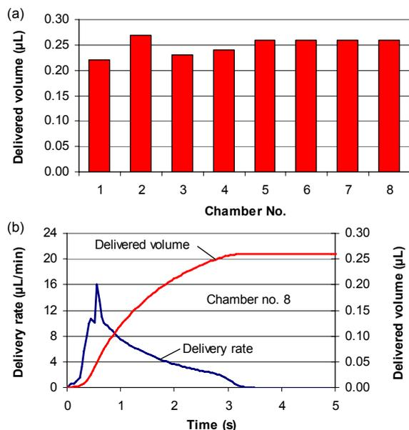
Figure 7: Representative delivery characteristics of a fluidic chip after individual heating with 225 mW for 10 s. (a) Delivered liquid volumes in consecutive order for one half of the device. (b) Transient delivery rate and delivered volume for chamber no. 8.
