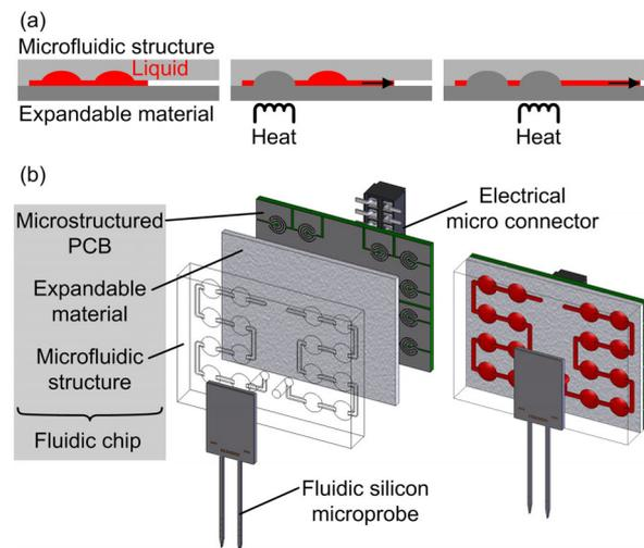
Figure 1: (a) Micropumping principle for liquid delivery. (b) Schematic drawing showing the different components of the NeuroMedicator.
