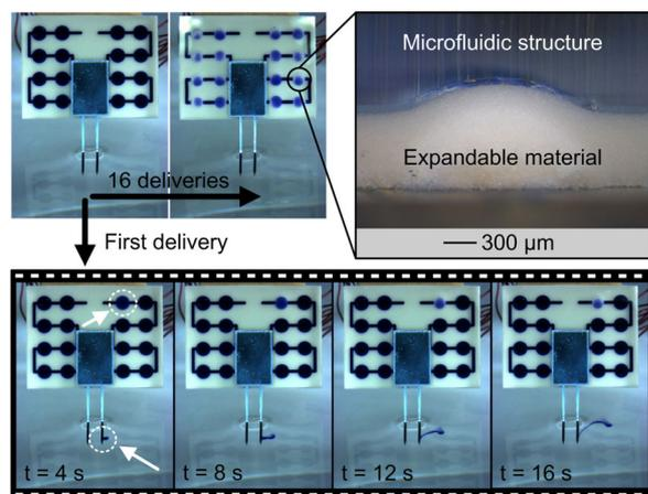
Figure 8: Transient actuation of an ink-filled NeuroMediator with the probe tips inserted into water. A cross section of an actuated chamber shows complete delivery.
