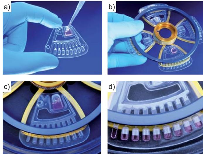
Figure 2: Process flow. (a) Loading of a chip with 165  $\mu\text{l}$  of a sample (here dyed water). (b) Loading of the carrier with four chips. (c) Carrier in Rotor-Gene. (d) Aliquoted liquid sample in reaction wells after centrifugo-thermopneumatic aliquoting.
