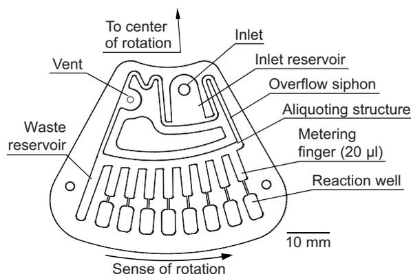
Figure 1: Schematic design of the microfluidic chip.
