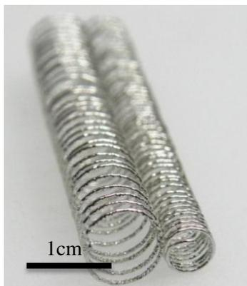
Figure 5: Coil like structures printed at 350°C metal temperature.
