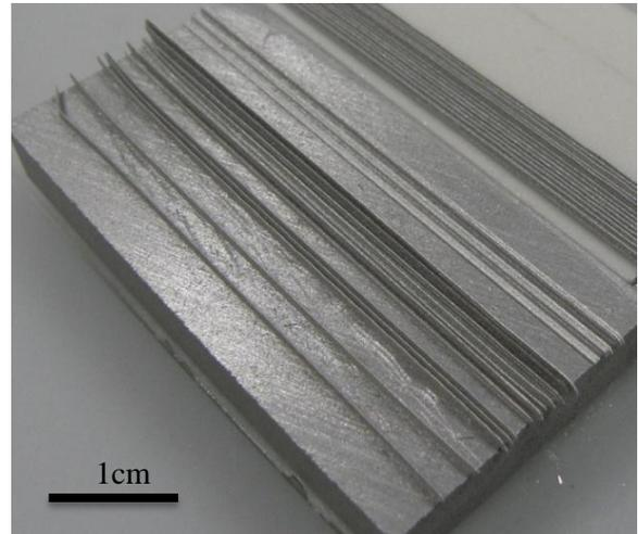
Figure 6: Walls printed at 350°C metal temperature on aluminum substrate.
