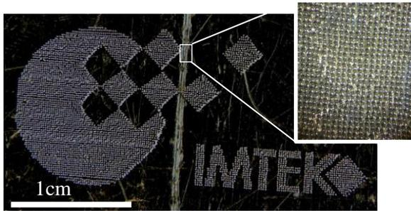
Figure 8: Printed IMTEK Logo, droplet diameter approximately  $80 \mu\text{m}$ .
