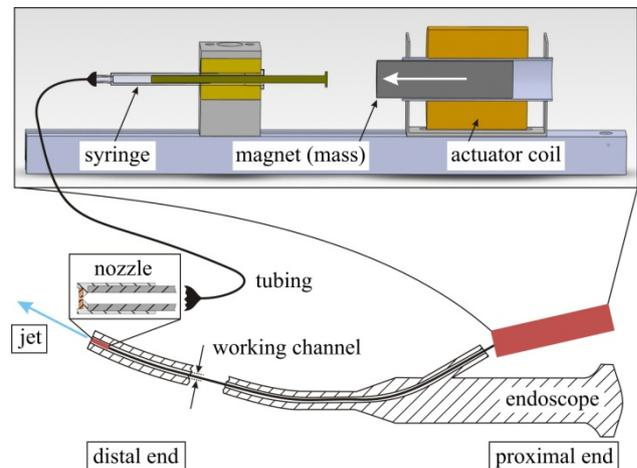
**Image 4:** Sectional drawing of the injection system for use through the working channel of an endoscope. A permanent magnet is accelerated and impacts with a defined momentum on the piston of a syringe.
