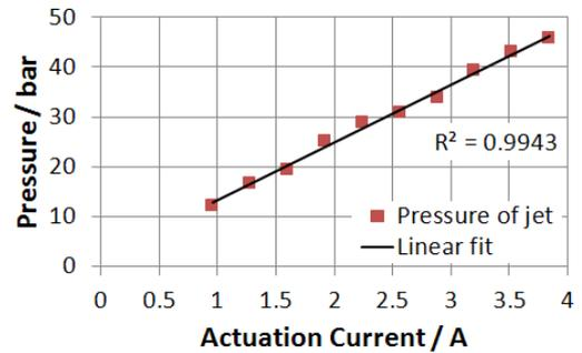
**Image 6:** The experimentally measured maximal pressure scales linearly with actuation current of momentum generator.
