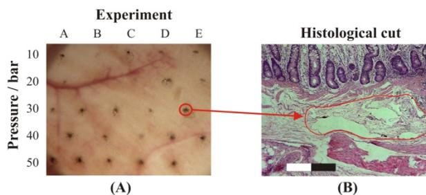
ed at a system pressure between 20 and 40 bar at valve opening times of 0.5 ms already reached the submucosa layer in most cases. Jets beyond 50 bar mostly lead to penetration of the target.
