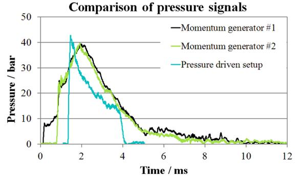
**Image 5:** Quantitative comparison of two measured pressure curves of ejected jets by using a driving current of about 3.2 A and the pressure driven setup, working with a high precision valve.
