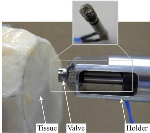
**Image 2:** Pressure driven setup with target tissue and Gyger Valve [7] in holder, which is the connection to BSP-Tubing
