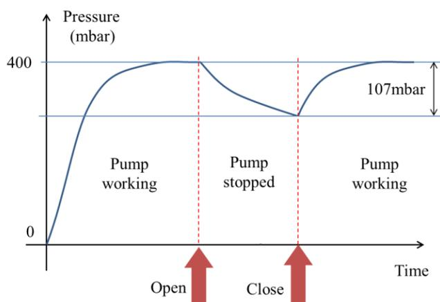
Figure 2: Typical signal during dispense (pressure difference 107 mbar). First the linear drive builds up the pressure by pushing the plunger into the syringe body. When the valve opens (first red arrow), the pressure (blue) drops until a certain pressure difference is reached; the valve is then automatically closed (second red arrow).
