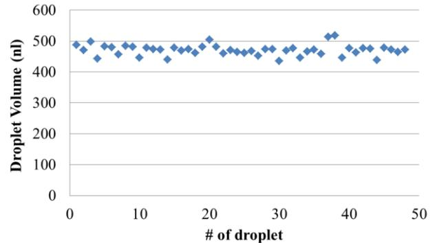
Figure 4: Results of 48 gravimetrically measured droplets of water at a mean volume of 470 nl and a standard deviation of 3.7%.
