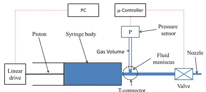
Figure 1: Schematic of the sensor controlled dispenser showing the different parts of the device.
