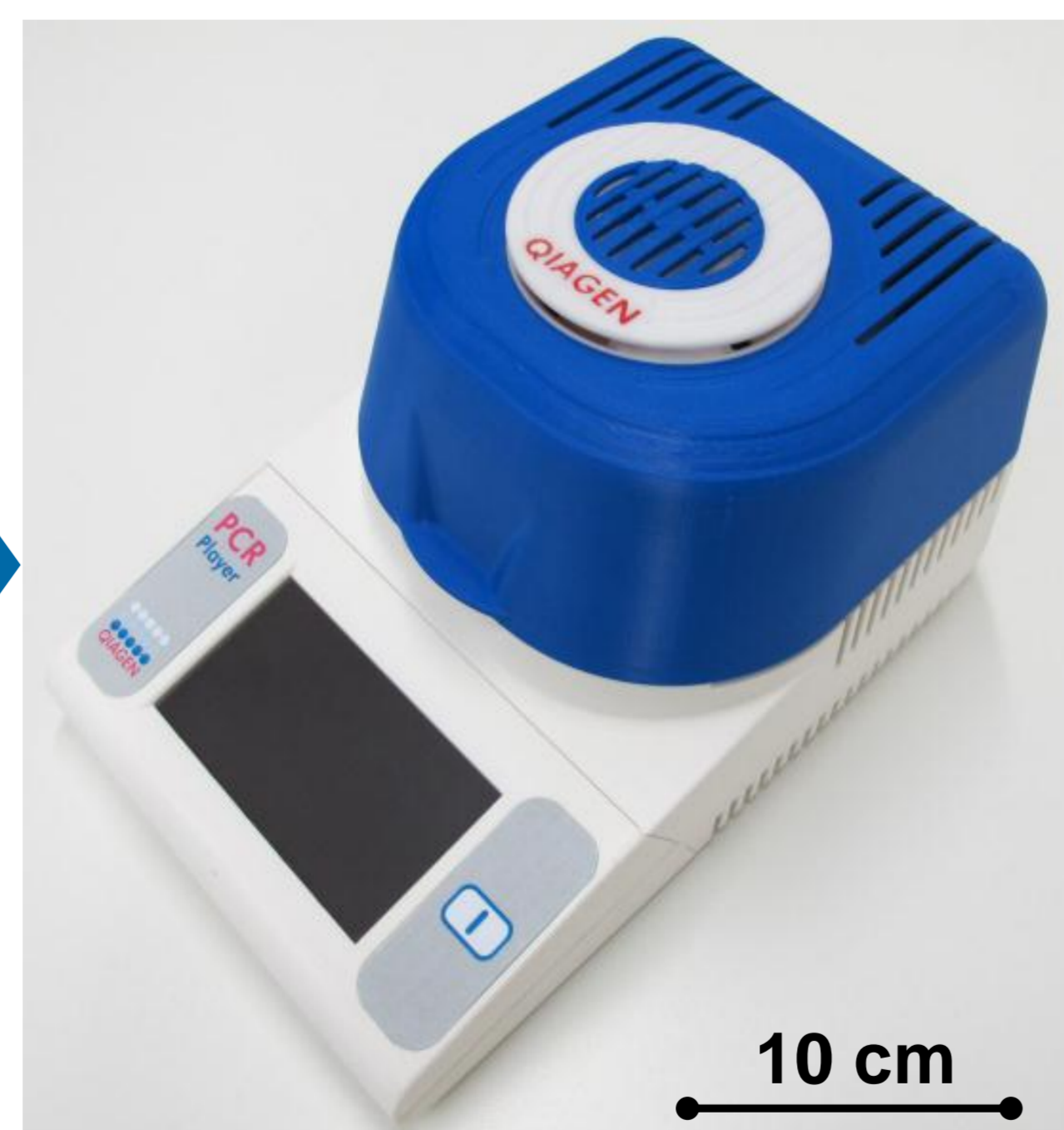
Fig.2 – LabDisk Player – A centrifugal processing device with integrated PCR-thermocycling chamber
