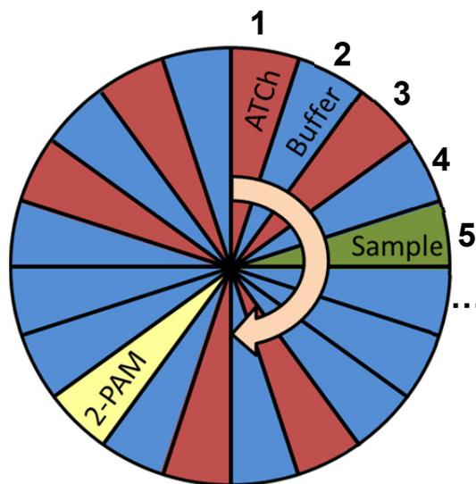
Figure 4: Order of reagents for one assay in the prefilled reagent module. The arrow indicates the start point and the rotational direction of the sensor. ATCh (red): Acetylthiocholine, substrate for the enzyme reaction; Buffer (blue) for washing the sensor; Sample (green): Milled cucumber; 2-PAM (yellow) pralidoxime, regeneration reagent. The numbers show the process steps for the ball-pen mechanism.
