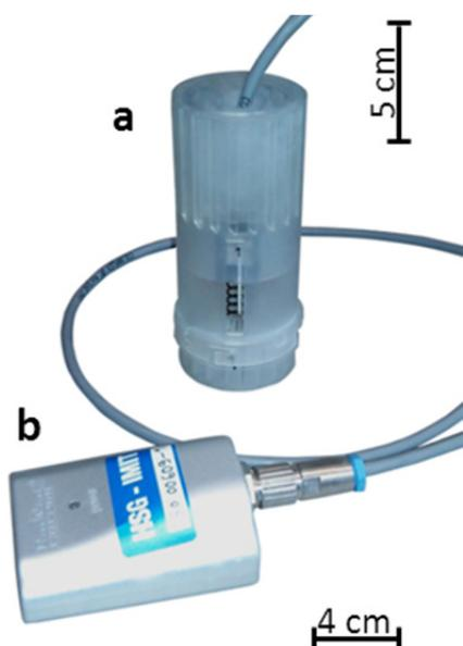
Figure 3: Prototype of assembled cartridge produced by stereolithography (a) and the potentiostat EmStat<sup>2</sup> (b).
