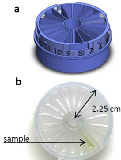
Figure 2: Reagent module as 3D-drawing (a) and as a prototype (b) filled with reagents and sample. For pre-storage of reagents, the module can be sealed by an easily removable foil like a yoghurt cup.
