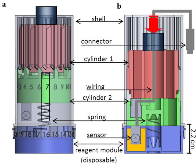
Figure 1: Cartridge for automated pesticide detection. The ball pen mechanism for rotating and dipping the sensor is realized by a shell, two cylindrical elements and a spring. a) Switching position: The spring is not compressed and the sensor does not contact reagents. B) Incubation position: The Spring is compressed, activated manually or by a single axis coordinator and the sensor is dipped into a reagent/sample for incubation.
