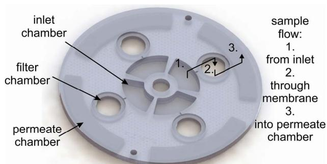
Figure 2: Microfluidic structure for on-disk enrichment of bacteria. The novel unit operation consists of three chambers: an inlet chamber at the upper side of the disk into which the sample is loaded, a filter chamber connecting the upper side of the disk to the lower side and a permeate chamber on the lower side collecting the permeate of the filtering process. Four enrichment structures fit on one LabDisk.
