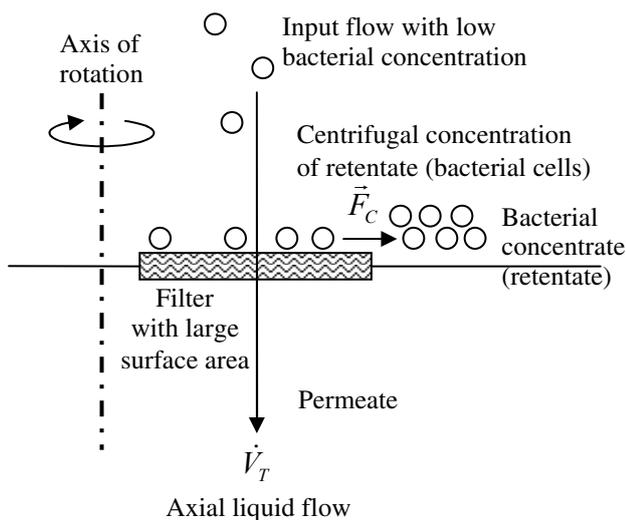
*Figure 1: Schematic of the axial centrifugal filtration approach. An input flow with low bacterial concentration is filtered axially. The retained bacterial cells are centrifuged radially outward to further concentrate the bacteria and to prevent filter clogging.*
