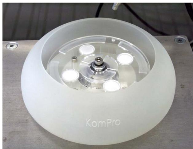
Figure 3: Photograph of the produced LabDisk carrying the axial filtration structures. Filters are inserted into the filter chambers by thermal bonding. The LabDisk is inserted into a receptacle which can be used to collect clean and filtered permeate when processing samples of large volumes. The receptacle can be connected to a larger vessel for storage of the larger fluid volumes.
