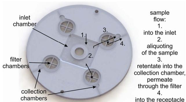
Figure 5: Microfluidic structure for continuous on-disk axial filtration of bacteria featuring one inlet chamber arranged circularly around the axis of rotation. A filter support structure is implemented inside the through holes of the filter chambers. Due to the centrifugal force, bacteria are transported radially outwards, across the surface of the filter into collection chambers. Permeate is continuously transferred to the receptacle.
