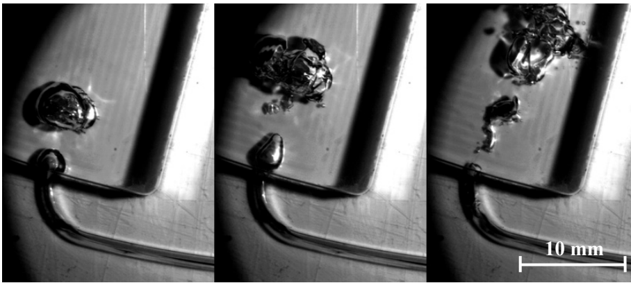
Figure 2: Oxygen bubble formation in a fluidic chamber filled with water. Each bubble is at a different state after ejection from the adjacent channel. The instability caused by centrifugal acceleration and subsequent separation in numerous small bubbles is clearly visible.
