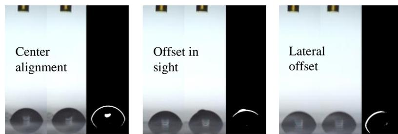
*Figure 2. Dispenser alignment validation from stroboscopic setup. Each subframe represents a series of single droplet injection: before-after-subtraction. A closed white semicircle indicates complete injection.*
