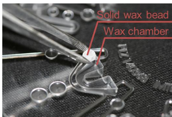
Figure 1: During fabrication of the centrifugal microfluidic COP cartridge, the CTP wax valve only requires a single and simple pick-and-place process of a solid wax bead into the wax chamber. Afterwards, the microthermoformed cartridge is sealed.
