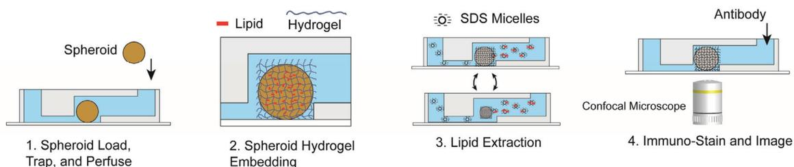
Figure 2: Process overview for optical clearing of spheroids on a microfluidic large-scale integration chip platform with (i) spheroid trapping, (ii) fixation and hydrogel embedding, (iii) lipid extraction and (iv) protein staining.
