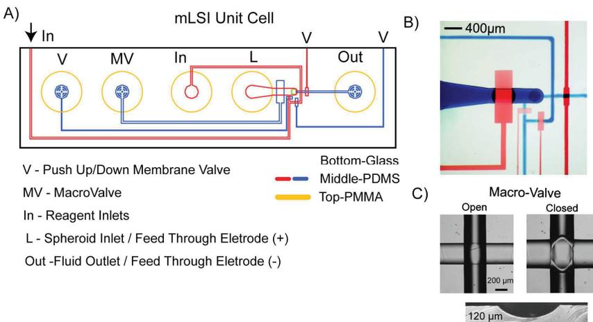
Figure 1: Design of the microfluidic large-scale integration chip platform. A) Flow logics of a unit cell, which can be arrayed on a mLSI chip. B) Real chip image. C) Example of a 'MacroValve', with a size of 360x360  $\mu\text{m}$  for spheroid loading.
