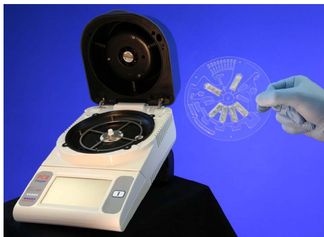
Figure 1: The LabDisk platform (former fluidic layout) with a portable point-of-care prototype LabDisk player for automation of all necessary assay and liquid handling steps.
