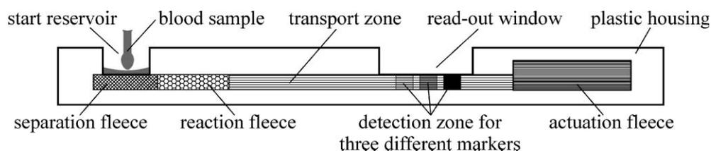
Fig. 1 Simplified cross section of a typical capillary driven immunoassay test strip.
