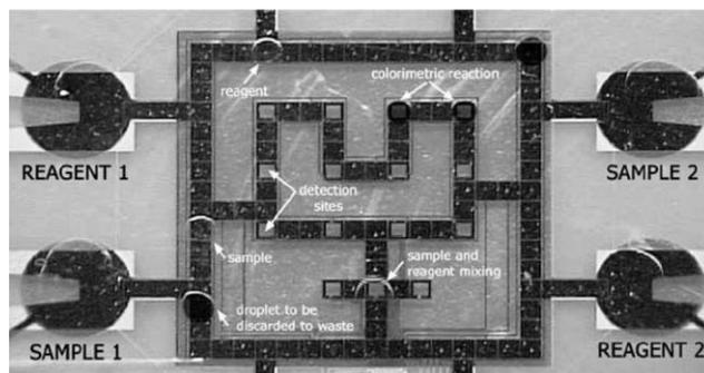
**Fig. 10** Integrated lab-on-a-chip architecture for a colorimetric glucose assay, based on the droplet based electrowetting platform. Four reservoirs with injection elements are connected to an electrode circuit, where the droplets are mixed, split and transported to detection sites for readout.<sup>123</sup> Reproduced by permission of the Royal Society of Chemistry.
