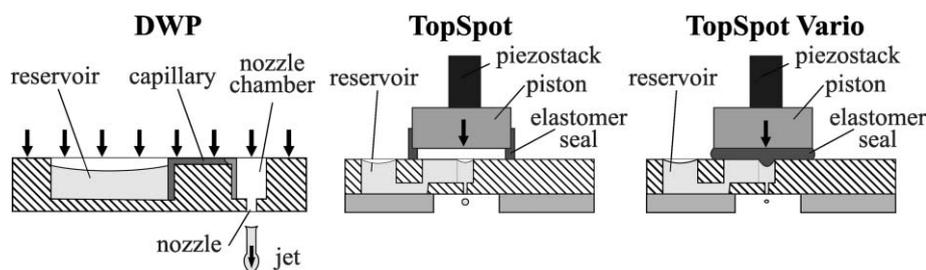
**Fig. 11** DWP: pressure based actuation for dispensing from 10 nL up to several  $\mu\text{L}$ , TopSpot<sup>®</sup>: pressure based actuation for dispensing volumes in the lower nL range, TopSpot<sup>®</sup> Vario: direct displacement principle *via* an elastomer for dispensing of volumes from 100 pL to 1400 pL.
