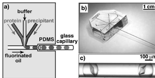
**Fig. 9** Microfluidic realization of a protein crystallization assay, based on the pressure driven droplet-based platform.<sup>109</sup> The protein and precipitation solution are continuously injected into one droplet of adjustable volume (a) and afterwards transported into a glass capillary for crystallization (b). Re-circulating flows inside the droplets enhance mixing and induce the crystallization process (c). (Reprinted with permission from ref. 109.)
