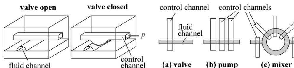
**Fig. 2** Construction of the main unit operations on the multi-layer PDMS based LSI platform. The NanoFlex™ valve as depicted on the left can be closed by applying a pressure  $p$  to the control channel. Therewith, microfluidic valves (a), peristaltic pumps (b) and mixing structures (c) can be designed.
