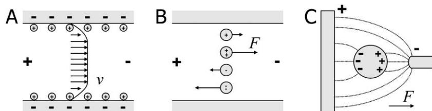
Fig. 6 Basic electrokinetic effects. A: Electroosmotic flow (EOF), B: electrophoresis (EP), C: dielectrophoresis (DEP).
