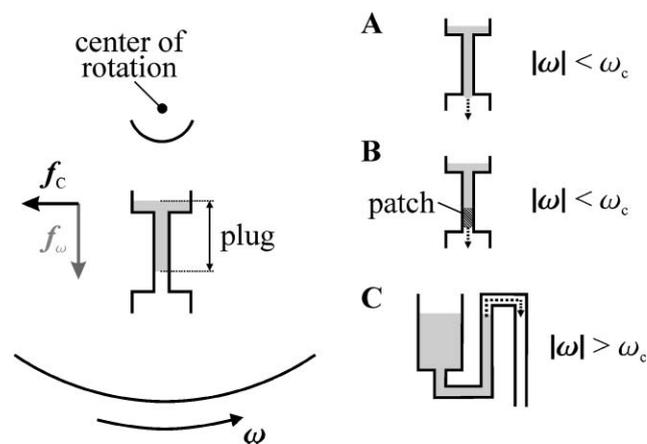
**Fig. 4** Principal centrifugal approach and schematic sketch of the three valving techniques on the centrifugal platform. (A) geometric capillary valve, (B) hydrophobic valve and (C) hydrophilic siphon valve.
