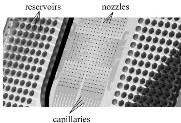
**Fig. 12** The TopSpot<sup>®</sup> technology combines the unit operations reagent storage (in top side inlet reservoirs), liquid transport (through capillary channels), metering and transfer *via* a free-flying droplet through the micronozzle as soon as the piezostack is actuated. The depicted TopSpot<sup>®</sup> 384 printhead features 384 dispensing units enabling the contact-free transfer of 384 different liquids onto planar substrates (microarrays).
