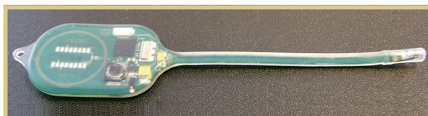
Figure 6. Fully implantable wireless sensor for the intracranial pressure monitoring system.
