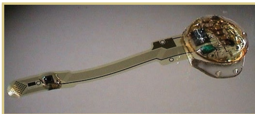
Figure 2. Retinal stimulator for the Healthy Aims retinal implant system. The electrode array is 4 \times 5.5 \text{ mm} , and the electronics is approximate 25 \text{ mm} in diameter.
