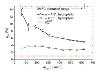
Fig. 6 Pump efficiency of a single-tapered channel plotted against the gas flow rate for different taper angles  $\alpha$
