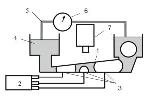
Fig. 3 Experimental set-up for the investigation of pump rates induced by moving gas bubbles in tapered channel structures. *I* tapered channel structure, 2 three syringe pumps, 3 three individual gas inlets, 4 reservoir, 5 tubing, 6 flow sensor, 7 camera
