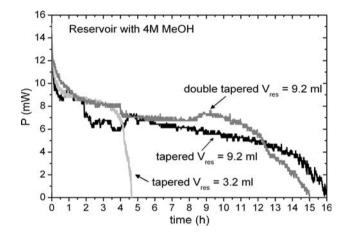
Fig. 11 Long-term performance of the fully passively operating DMFC for different reservoir fillings and for different channel types at ambient temperature ( $T = 23^{\circ}$ C)
