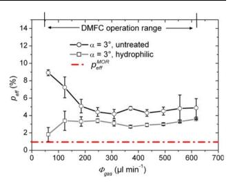
Fig. 7 Pump efficiency of a single-tapered channel with and without surface treatment plotted against the gas flow. The bottom channel surfaces are covered with a porous transport layer (PTL) to simulate configurations similar to DMFC operation
