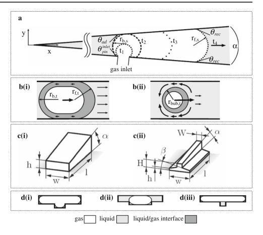
*x*-direction, thus, the deformed bubbles exhibits interfaces with different curvatures at the front and the back of the bubble which leads to a pressure difference over the whole bubble, according to the law of Young–Laplace.
