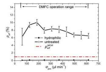
**Fig. 9** Pump efficiency of a double-tapered T-shaped channel as shown in Fig. 3b plotted against the gas flow rate. In the untreated configuration, the channel is covered with a porous transport layer (PTL) to simulate more realistic DMFC operation conditions
