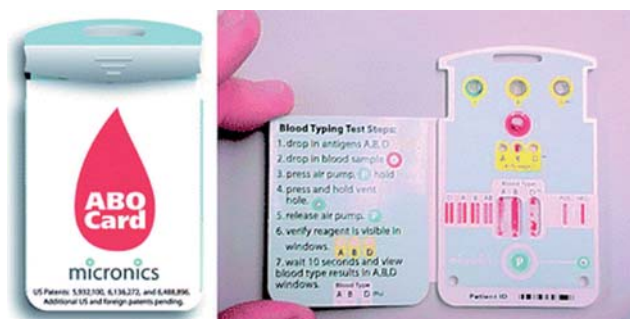
Fig. 27 Disposable device for ABO blood typing developed by Micronics, Inc. 44 All fluids are moved and aliquoted through capillary force and manual on-card bellows pumping. Reagents and sample are mixed passively along laminar flow diffusion interfaces in microchannels. The result visible in the viewing window indicates blood type A, Rh positive. Figure and parts of caption reproduced by permission of The Royal Society of Chemistry.
