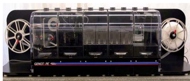
Fig. 25 Instrument by Douglas Scientific for continuous reel-to-reel handling of array tape. 30 The wells can be loaded, dried and sealed prior to thermocycling. Figure reprinted with permission from Elsevier.
