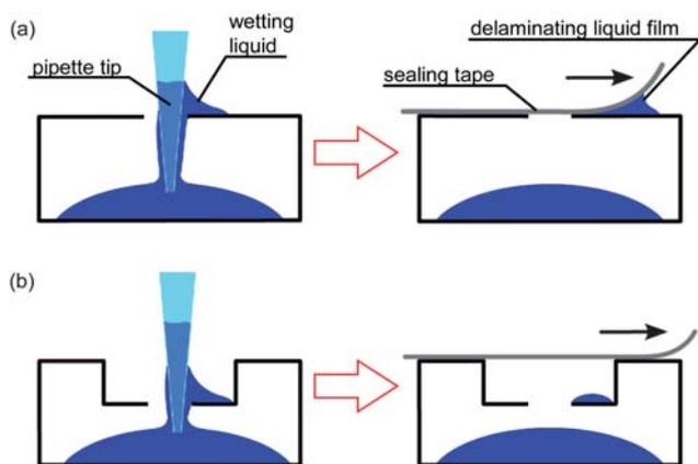
**Fig. 4** Method for sealing inlets after insertion of highly wetting liquids (not to scale). (a) Sealing tape is wetted by remaining liquid and can thus delaminate. (b) The novel inlet design prevents wetting of sealing surfaces and allows robust sealing of inlet holes.
