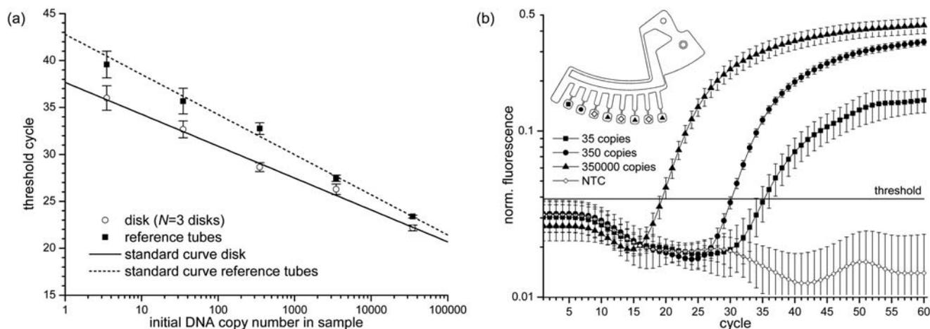
**Fig. 6** Results of real-time PCR on a foil disk. (a) Threshold cycles and standard curves of 3 foil disks with varying copy numbers and a reference in standard tubes. Amplification of less than 10 copies per reaction is feasible. (b) Examination of cross-contamination across the reaction wells. High amounts of DNA do not contaminate adjacent wells with NTCs as NTC signals remain below threshold.
