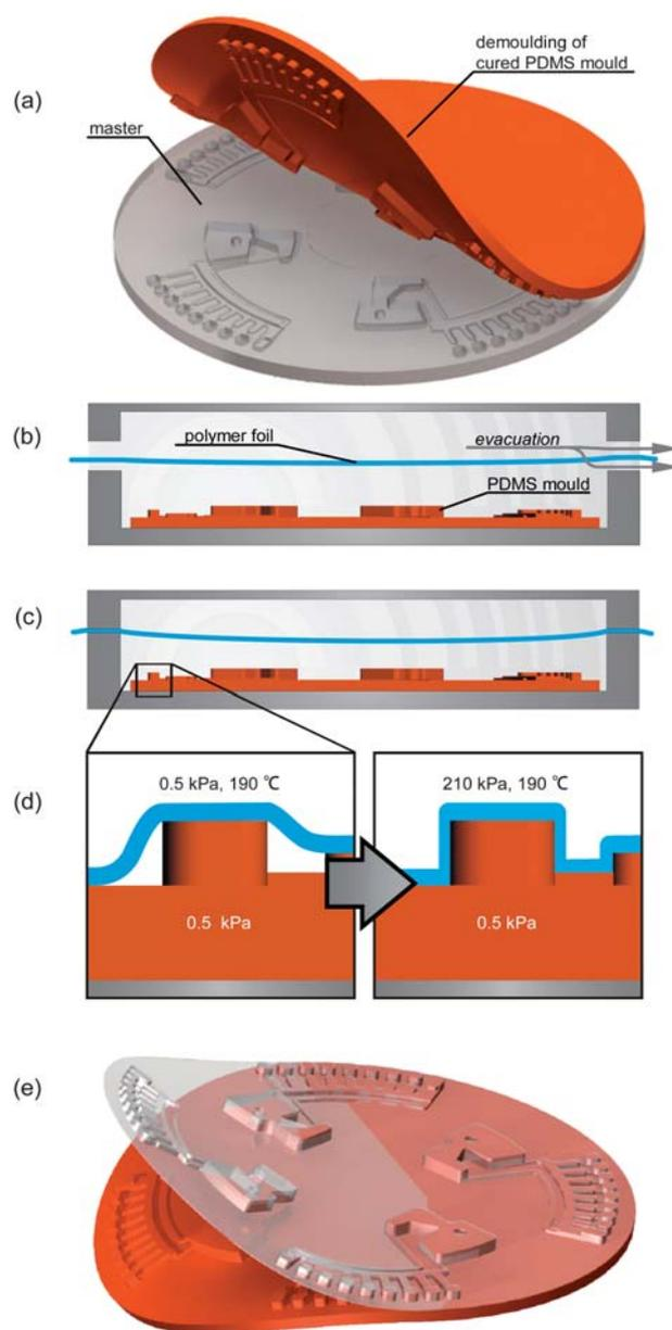
**Fig. 3** Process flow for the formation of COP foils. (a) Fabrication of the PDMS mould; (b) assembly in a modified hot embossing machine and evacuation; (c) clamping of the foil in vacuum; (d) moulding of the foil through application of a pressure difference at moulding temperature; and (e) demoulding after cooling, venting and opening of the process chamber.
