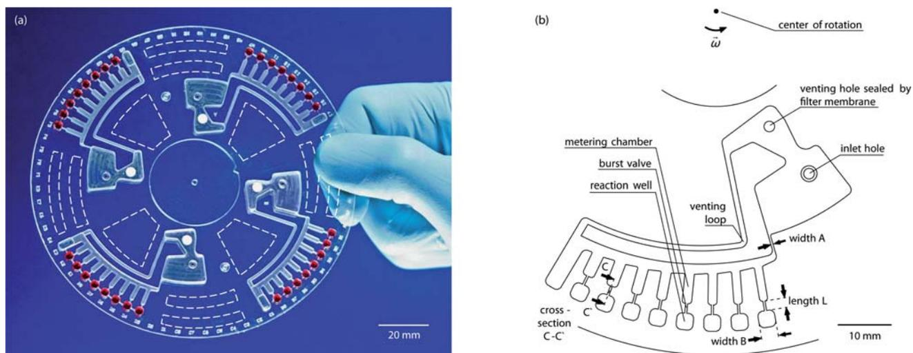
**Fig. 1** Design of the foil cartridge. (a) Photograph of a foil disk (reaction wells are highlighted with a dye, contours of through holes for air flow are indicated as dashed lines); and (b) CAD drawing of a segment with microfluidic elements, sense of rotation  $\omega$  and characteristic geometries (widths A and B, length L, and cross-section C-C').
