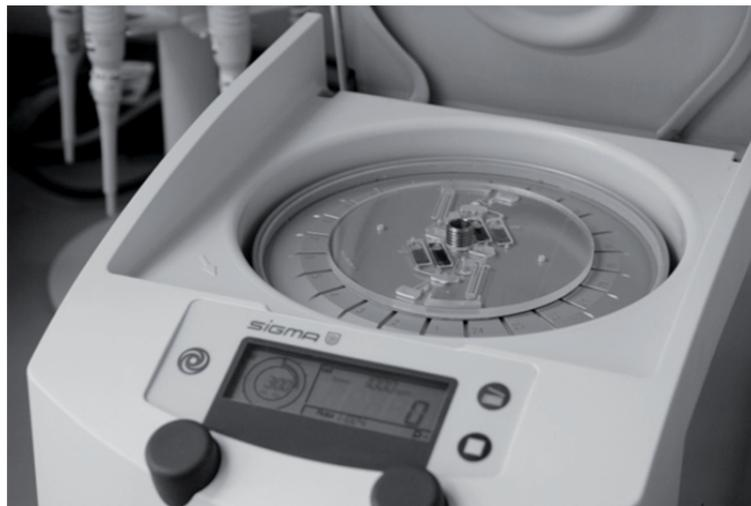
Figure 2. Microfluidic cartridge for DNA-Extraction operated in a standard laboratory centrifuge.
