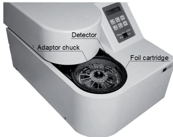
Figure 4. Microfluidic cartridge for genotyping processed in a slightly modified Rotor-Gene thermocycler
