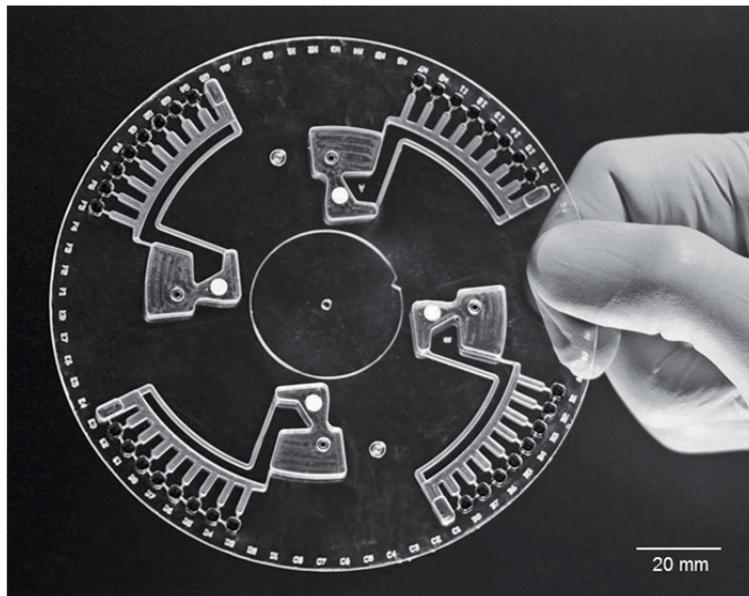
Figure 3. Microfluidic cartridge for genotyping of DNA. Up to four samples can be processed independently in each disk. On the outer diameter are four separate structures comprising eight reaction wells (highlighted with a dye for better visibility) and a reservoir for waste liquid.
