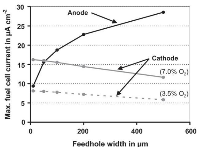
**Fig. 3.** Influence of feedhole width on the maximum reactant flux at the electrodes (as indicated in the figure) sustainable by a given feedhole geometry, expressed as maximum fuel cell current density according to Eqs. (5) and (6).
