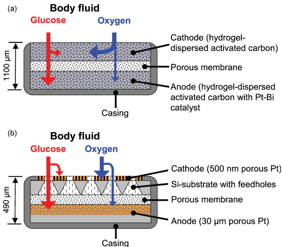
**Fig. 1.** Comparison of two construction concepts for abiotically catalyzed glucose fuel cells. (a) State-of-the-art approach with hydrogel-dispersed activated carbon electrodes [6]. (b) Binder-less concept presented in this work, employing a thin-layer platinum cathode deposited on a silicon substrate with micro-machined feedholes, and a self-supporting platinum anode.
