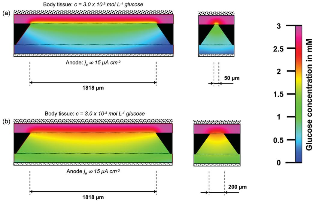
Fig. 4. Steady-state glucose concentration profiles at a current density of  $15 \mu\text{A cm}^{-2}$ . (a)  $50 \mu\text{m}$  wide feedhole. (b)  $200 \mu\text{m}$  wide feedhole. Shown are cross-sections in the center of the unit cell, both along the feedhole's width ( $w_f = 50$  and  $200 \mu\text{m}$ ) and length ( $l_f = 1818 \mu\text{m}$ ).
