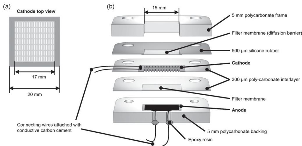
**Fig. 6.** Fuel cell construction details. (a) Top view of the permeable cathode. The light-colored area represents the slit-array onto which the catalyst is deposited. (b) To-scale cross-sectional view of the binder-less glucose fuel cell assembly. See text for explanations.
