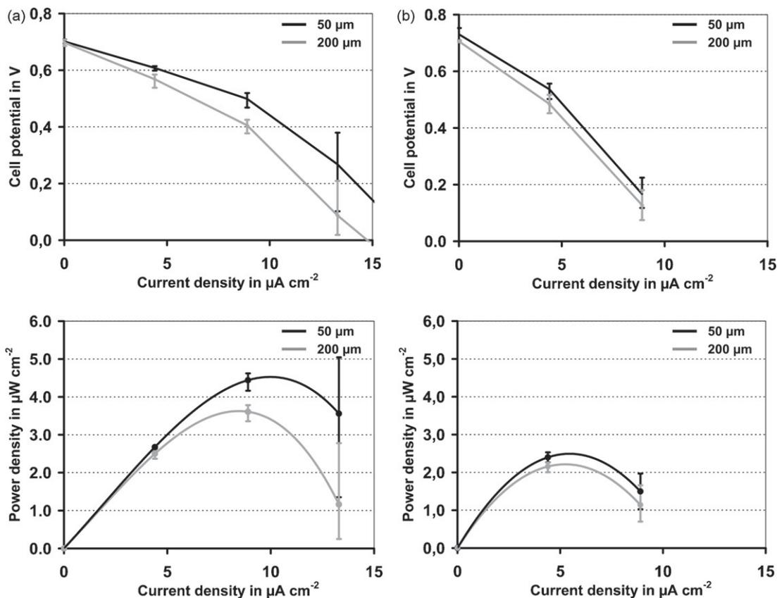
Fig. 8. Polarization curves of complete fuel cells with 50 and 200  $\mu\text{m}$  wide feedholes (as indicated). Recorded at (a) 7.0% oxygen saturation and (b) 3.5% oxygen saturation in the testing solution. Average of triplicate experiments, bars represents maximum and minimum values.
