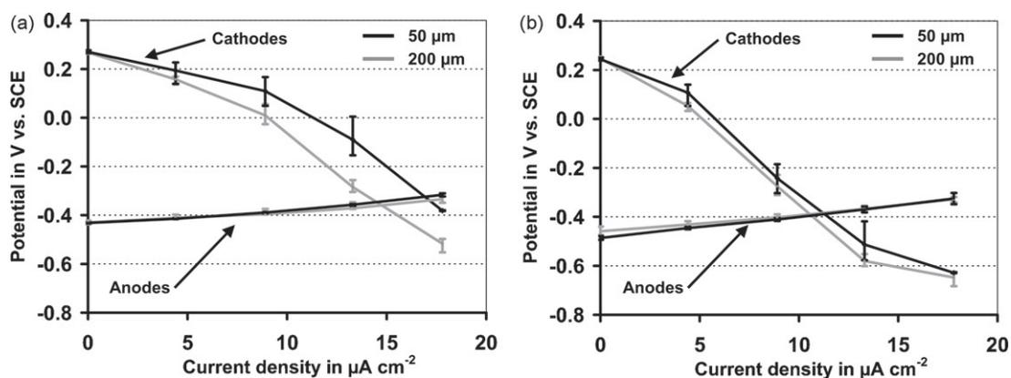
**Fig. 7.** Individual polarization curves of anode and cathode of operating fuel cells with 50 and 200 μm wide feedholes (as indicated). Recorded at (a) 7.0% oxygen saturation and (b) 3.5% oxygen saturation in the testing solution. Average of triplicate experiments, bars represents maximum and minimum values.
