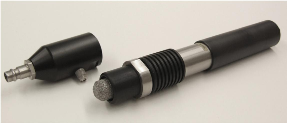
**Figure 8.** Photograph of the realized sensor system. The sensor system on the right is portable and intended to measure in free atmosphere. The sensor system can be equipped with an adapter shown on the left. This adapter contains a quick connect for connecting the sensor system to and measuring in tubing systems. An exhaust throttle allows gas to flow through the connected adapter.
