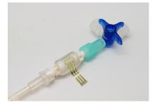
The aim of this project is to develop novel sensor technologies – based on capacitive concepts – by which flow rate and composition of fluids can be continuously and instantaneously monitored. It should be investigated how mixtures of liquids affect the output signal of a given sensing element, and therefore which parameters of the mixture of liquids can thus be measured.
