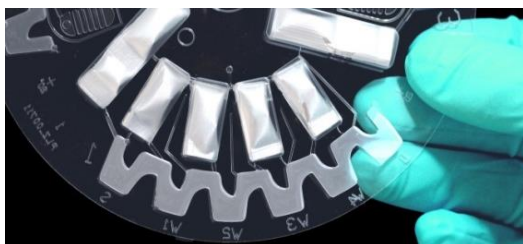
Figure 3: Stickpacks for liquid reagent pre-storage and release on demand inserted into a LabDisk.
