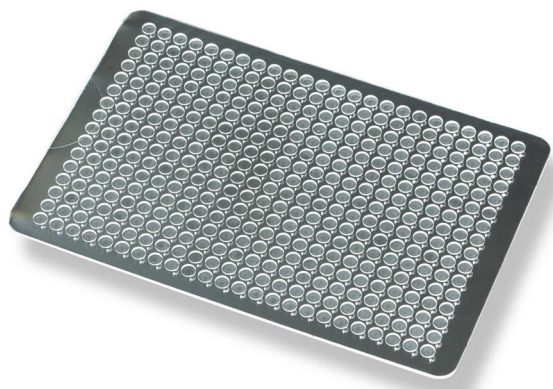
Fig. 1: Photograph of a 384-unit DWP made of COC (TOPAS 5013/size 120x80 mm 2 ; pitch: 4.5 mm).
