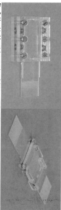
Fig. 2. Hand-held protein array translators consisting of 2 microscope slides and incubation chamber made of laser-cut self-adhesive polyester foil: prototypes for top priming with liquids (a) and lateral priming (b) of the cell free expression system.
