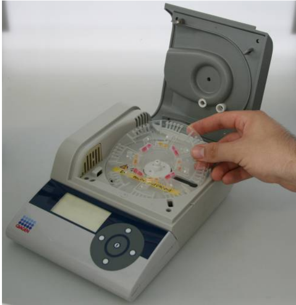
Figure 1: Portable diagnostic system for point-of-care applications comprising a disposable LabDisk for the nucleic acid based detection of pathogenic microorganisms and the immunoassay based detection of toxins, as well as a centrifugal processing device.
