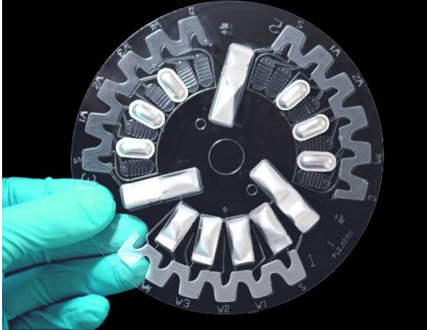
Figure 2: Disposable test carrier for immunoassay: reagents are stored in aluminium pouches. If centrifugal force is applied, the pouches burst due to the increased hydrostatic pressure of the liquid.
