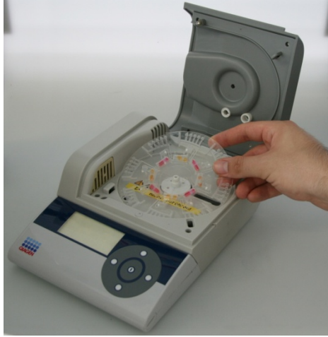
Fig. 1. The portable LabDisk Player. Integrated magnets can be used for the automated control and manipulation of magnetic beads e.g. for nucleic acid purification or bead based immunoassays
