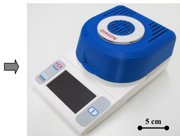
Figure 2 – LabDisk Player prototype enabling full process control (frequency, acceleration, thermocycling, fluorescence read-out)
