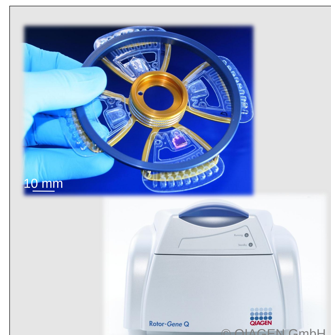
GeneSlices as Microfluidic Apps for multiplex PCR in standard Rotor-Gene.
