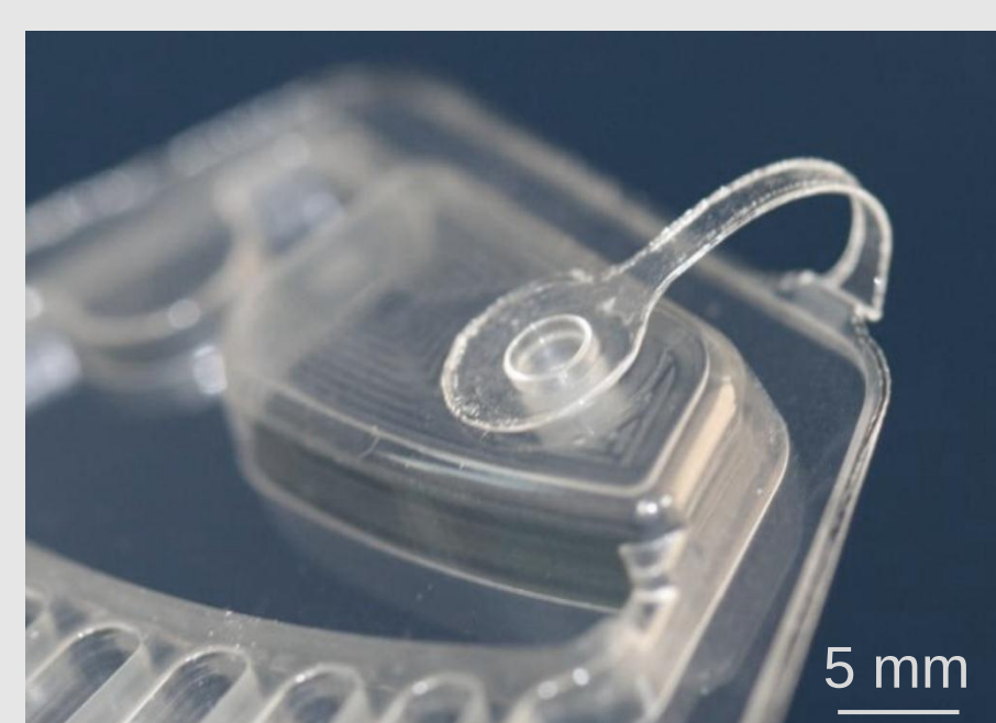
Closable sample inlet, monolithically fabricated by microthermoforming.
