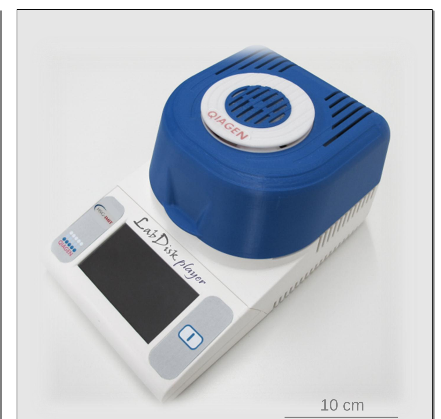
LabDisk processing device for spinning, thermocycling and real-time detection.
