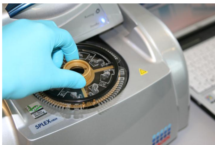
Figure 1: Microfluidic Apps for nested PCR feature low contamination risk in a self-contained Lab-on-a-Chip system, which can be processed in an unmodified standard laboratory real-time PCR thermocycler (Rotor-Gene Q, Qiagen, Germany). A special rotor holder enables insertion of four GeneSlices per run.
