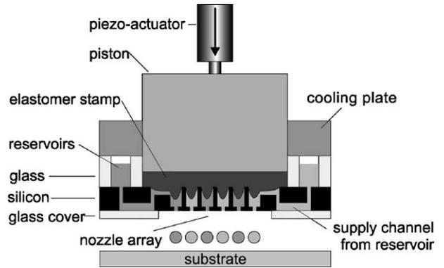
Fig. 3. Schematic of the elastomer deformation into printhead channels displacing the reagents.
