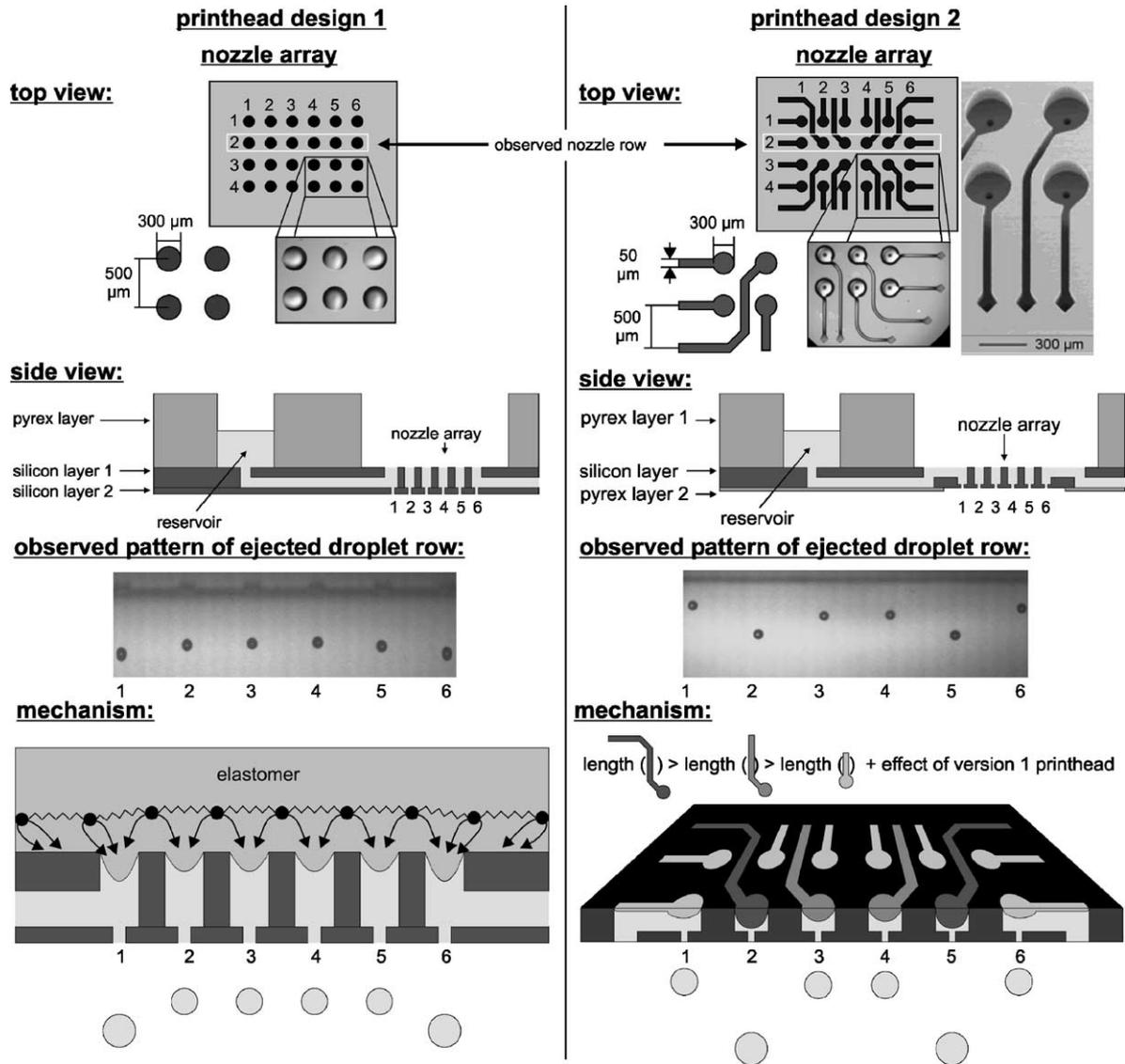
Fig. 6. The two investigated nozzle array designs that were investigated towards droplet homogeneity dependent of nozzle array type two different patterns of ejected droplets were observed.
