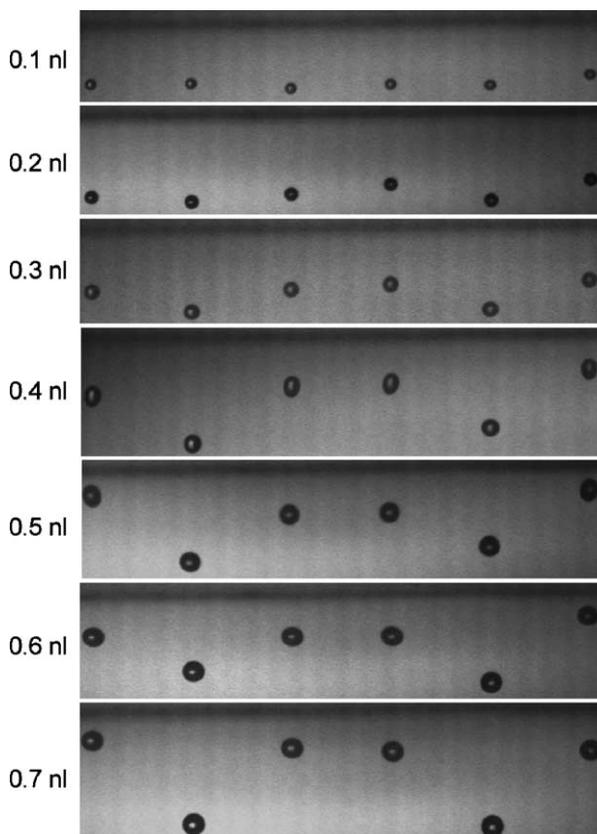
Fig. 7. Observed pattern of an ejected droplet row.
