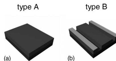
Fig. 8. Investigated stamp geometries: (a) flat elastomer-stamp; (b) spacer directly adjacent to the rubber stamp.
