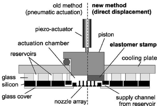
Fig. 2. Schematic of the old method based on air compression (left) and the new method based on direct displacement (right).
