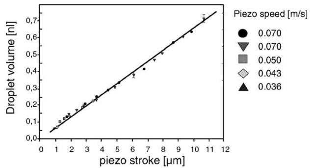
Fig. 4. The ejected droplet volume (nl) vs. piezo stroke (µm).
