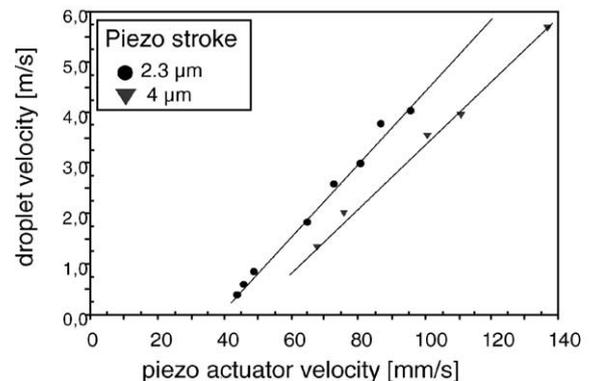
Fig. 5. Influence of the piezo speed ( $10^{-3}$  m/s) on the droplet speed (m/s).
