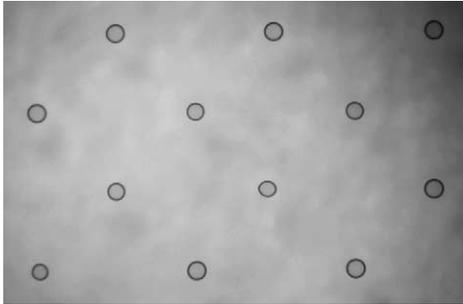
Fig. 9. Water and black ink are printed in a checkerboard pattern to demonstrate the absence of cross-contamination.
