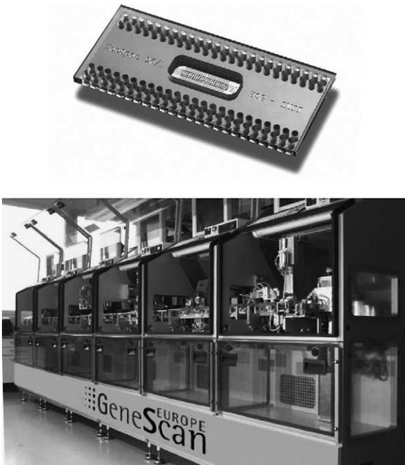
Fig. 1. Production line based on TopSpot-technology, spotting up to 1.440 different reagents at a throughput of 300 biochips/h, operated at Genescan Europe AG, Freiburg (D). Top: the 96 channel printhead.
