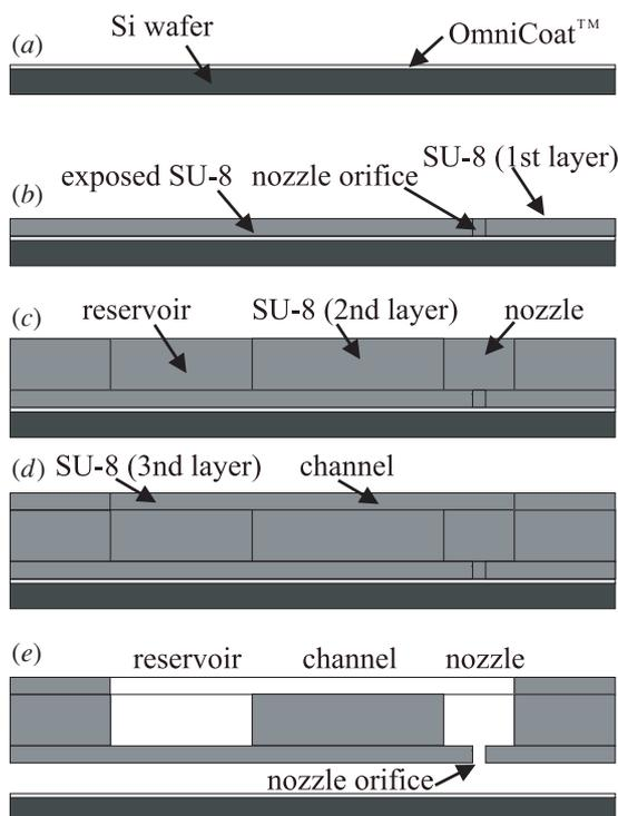
**Figure 4.** Description of the SU-8 lift-off process for the fabrication of the DWP<sup>TM</sup> (see text for details).
