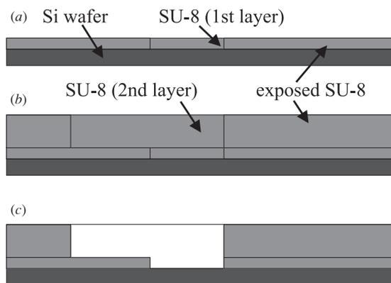
**Figure 1.** Principle of the multilayer SU-8 process: (a) first layer prebaked, patterned and postbaked, (b) second layer prebaked, patterned and postbaked, (c) simultaneous development (see text for details).
