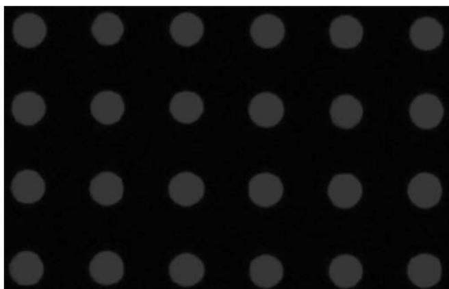
**Fig. 4** Fluorescent image of 1  $\mu$ M Cy3-labelled 20-mer oligonucleotide spotted in SSC buffer. Spot size 209  $\mu$ m, CV<2%; integral intensity of the complete array has a CV<5%, for all 24 spots
