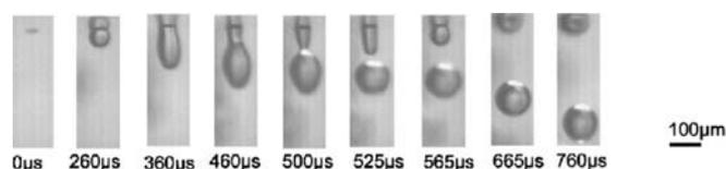
**Fig. 3** Stroboscopic observation of droplets (3×SSC buffer). Droplet size of 125  $\mu\text{m}$  with a CV below 1%
