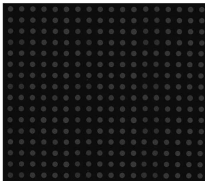
**Fig. 5** 4×3 arrays with Cy3-labelled Donkey anti goat IgG (0.66 mg L) in 1xPBS on ArrayLink hyphob. Coefficient of variation of the signal intensity below 4%
