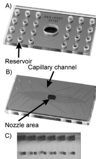
**Fig. 1A–C** The TopSpot printhead with 24 channels consisting of reservoirs, located on the outer rim. Each reservoir is connected to one nozzle through a capillary channel: **A** top view, **B** bottom view, **C** ejected droplet array
