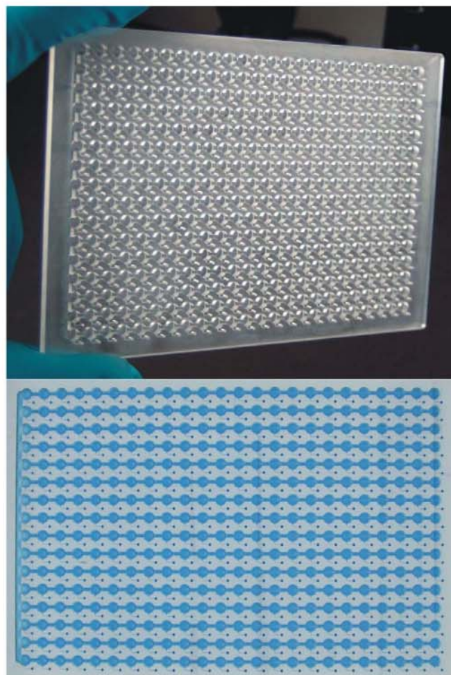
Figure 8. Bulk reagent dispenser DWP with 384 \times 1 \mu\text{L} dispensing volume made by micromilling in PMMA.
