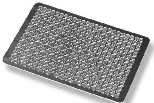
Figure 6. 384-unit DWP made by high-speed micromilling of COC.
