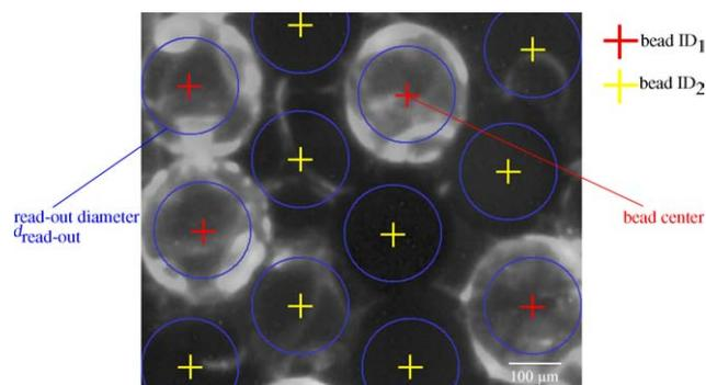
Fig. 7. Evaluation of the fluorescence signal. The assay result for each bead ID is measured by averaging the fluorescence signal within a circle of  $d_{read-out} < d_{bead}$  around the bead center for all beads of a certain ID.
