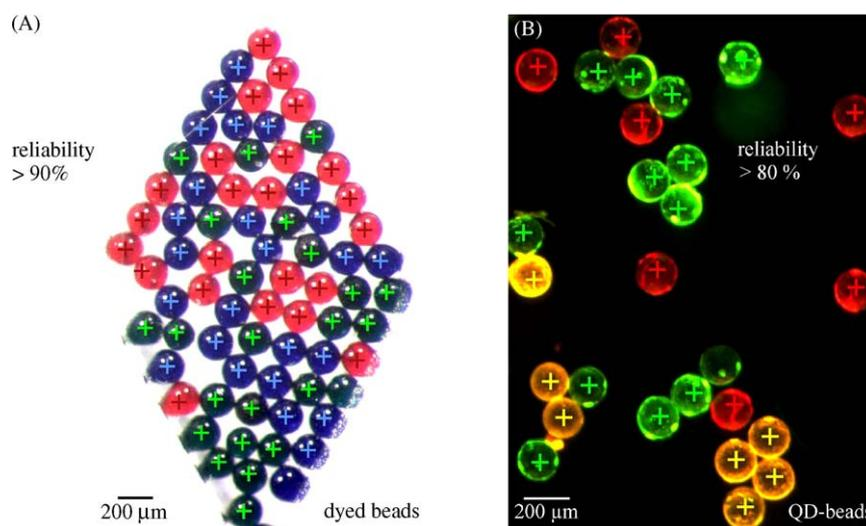
Fig. 6. Results of the image-processing routine for the evaluation of the bead ID. The localized bead centers are marked by a cross, where the assigned IDs are denoted by their color. (A) For the dyed beads, a reliability of higher than 90% can be achieved. (B) For the QD-beads, due to the inhomogeneity of the luminescence color over the bead surface, the reliability is reduced (slightly above 80%).
