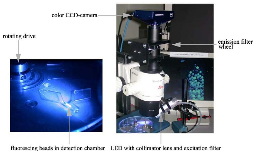
Fig. 3. Laboratory setup for the multiplexed assay. Fluorescing beads are aggregated in the detection chamber of the disk on the rotating drive. The beads are excited with a blue LED which features a collimator lens and an excitation-filter. The emitted fluorescence intensity is detected with a color CCD-camera after it passes the emission filter fixed in the emission filter wheel.
