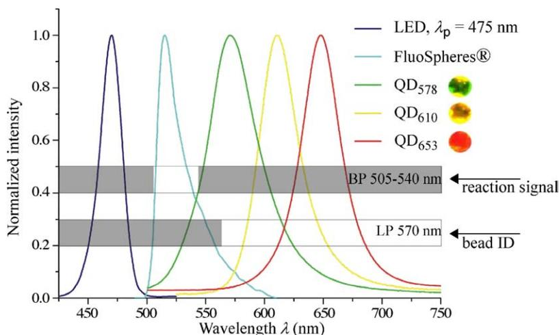
Fig. 2. Spectral distribution of the excitation source ( $\lambda_p = 475$  nm), the fluorescent label (FluoSpheres®), three types of QD-Beads (QD 578 nm, QD 610 nm, and QD 653 nm), and the applied filters (BP 505–540 nm and LP 570 nm).
