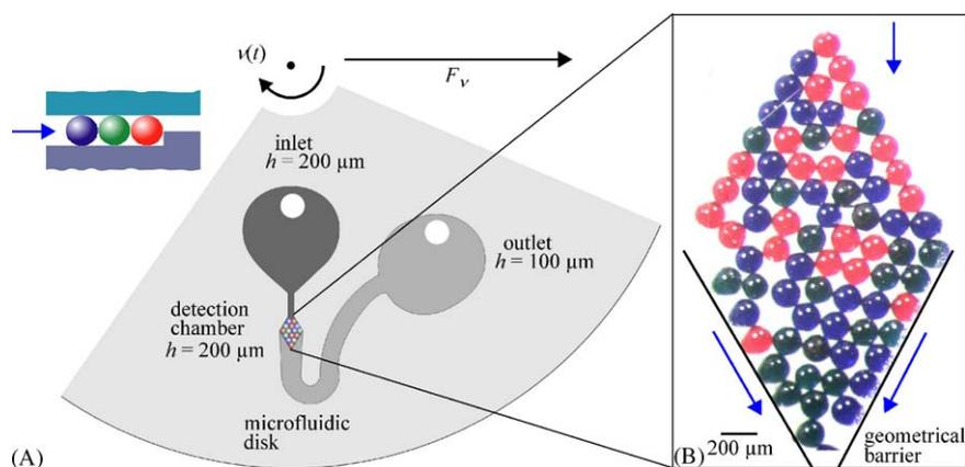
Fig. 4. (A) The chip which follows the format of a compact disk (CD) features only passive microfluidic elements: an inlet chamber ( $h = 200 \mu\text{m}$ ), a detection chamber ( $h = 200 \mu\text{m}$ ), and an outlet drain ( $h = 100 \mu\text{m}$ ). Flow rates and incubation times are controlled by a centrifugal frequency protocol  $\nu(t)$ . (B) In a preparative step of the sealed disk, the beads are aggregated in form of a periodic monolayer at a geometrical barrier.
