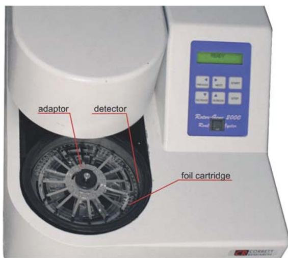
**Fig. 2** Assembly of the microfluidic foil cartridge in the modified centrifugal thermocycler Rotor-Gene 2000 (open top cover position).
