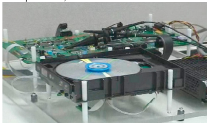
Fig. 5. DVD with microfluidically integrated hematocrit testing structures in DVD drive with modified firmware (figure according to [6]).
