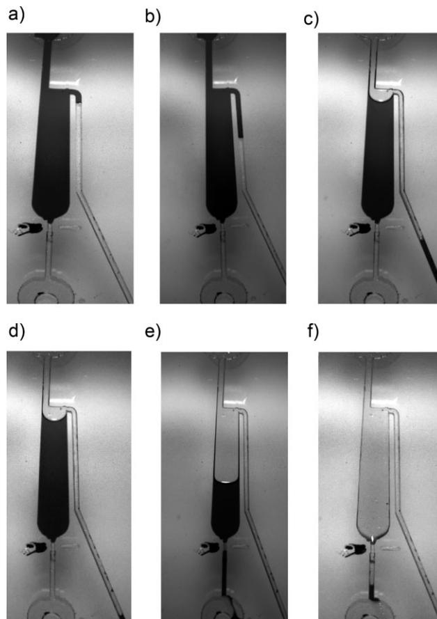
**Figure 10.** (a) Filling of a reservoir and channel on a disk using a dyed water solution (b) – (d) overflow of excess solution; (e) – (f) draining of 10 nL of solution at a spin speed beyond the critical burst frequency of 20 Hz.
