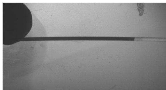
Figure 6. Optical image showing the wetting of only in the PEOx modified areas of the microfluidic channel.
