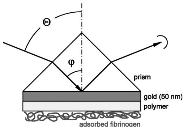
**Figure 2.** Schematic description of SPR set-up used for the protein adsorption experiments.
