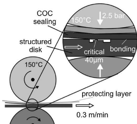
Figure 4. Schematic description of the set-up used for the lamination process.
