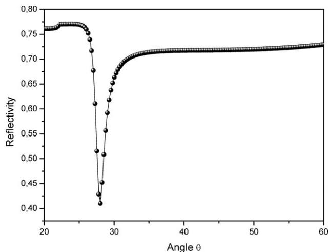
Figure 7. A typical reflectivity curve obtained in the SPR experiment on a 14 nm thick PMMA film on a gold coated lanthanum substrate (solid circles – experimental data; line – fit).
