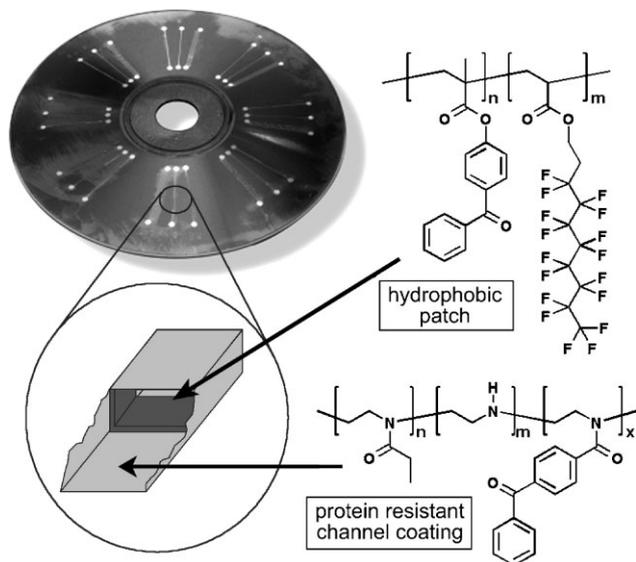
**Figure 1.** Schematic description of the surface modification of microfluidic channels.
