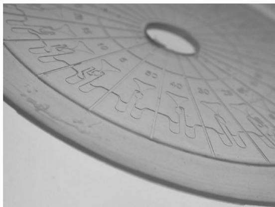
Figure 3. Optical image of microfluidic channels embossed into a CD consisting of polyethylene-co-norbornene.
