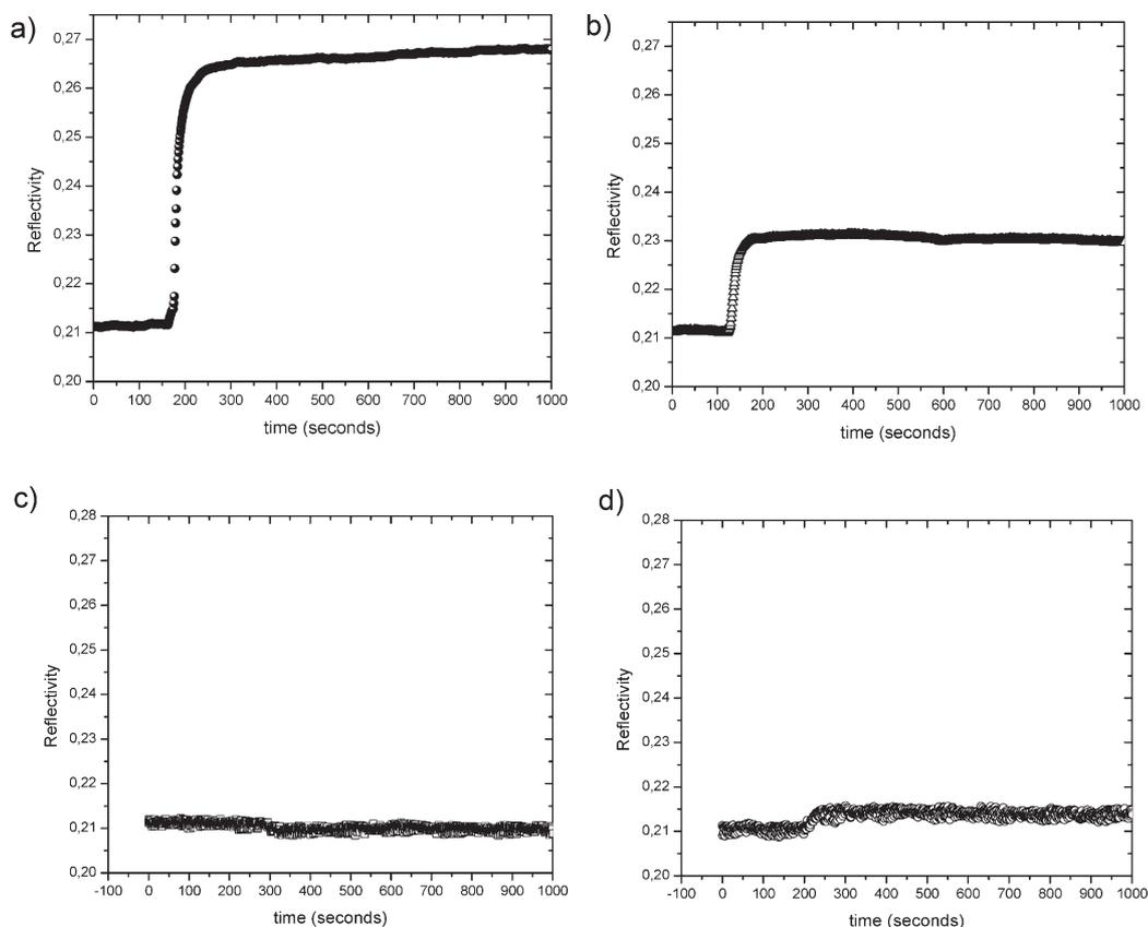
**Figure 8.** Measure of change in reflectivity with time in SPR experiments monitoring the adsorption of fibrinogen on (a) PMMA (b) PPFA (c) PEOx (d) PEG-thiol.
