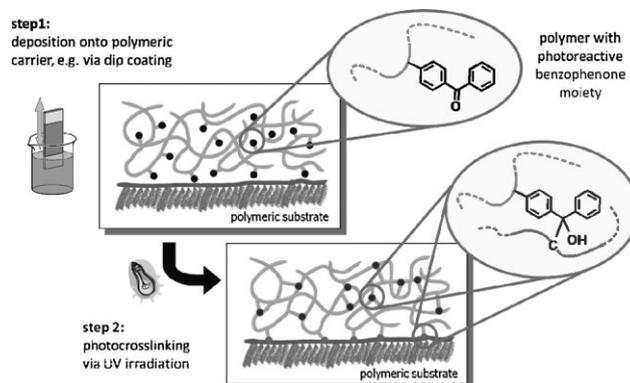
Figure 5. Schematic description of the photocrosslinking reaction that occurs between the photoactive benzophenone groups within the polymer and the polymeric substrate upon irradiation.
