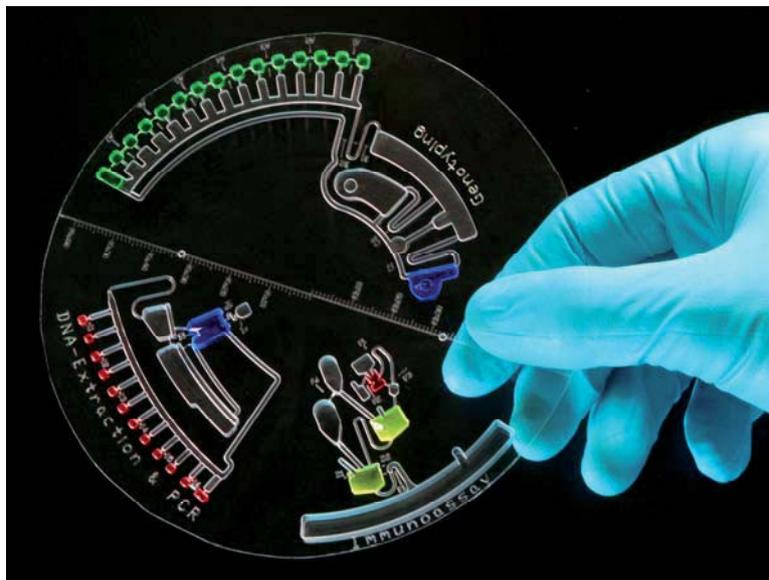
**Fig. 1.** Foil based test carrier containing thermoformed designs for real-time PCR analysis and immunoassays. Pre-stored reagents, reaction wells and read-out structures are highlighted with ink.
