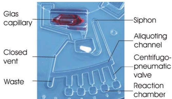
**Fig. 2.** Photograph of the thermoformed Lab-on-a-Chip test carrier for the detection of pathogens. The foil-based disc features a chamber with a glass capillary containing 50  $\mu\text{L}$  buffer for RPA and a chamber with a lyophilisate. A capillary siphon and a centrifugo-pneumatic valve are integrated for fluid control. An aliquoting structure splits the 50  $\mu\text{L}$  buffer into 5 x 10  $\mu\text{L}$ .
