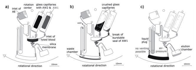
Figure 1. Microfluidic principle. a) Filling levels before rotation and uncrushed glass capillaries containing washing buffers AW1 and AW2; b) break of burstable seal of AW1 and centrifugation of AW1 into the waste chamber; subsequent automatic release of AW2; c) elution step after breakthrough of burstable seal of AE and blocking the switch channel by a liquid plug. Thereby the elution buffer AE is guided into the elution chamber, after collecting the purified DNA from the silica solid phase.
