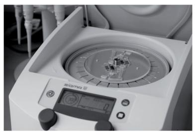
Figure 2. Microfluidic cartridge for DNA-Extraction operated in a standard laboratory centrifuge.
