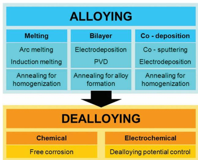
**Figure 22.** Optional pathways for the fabrication of nanoporous platinum by dealloying.
